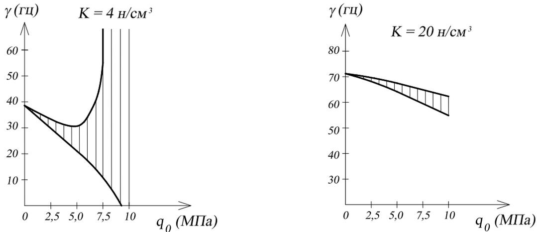
**Fig. 4 and 5. The regions of dynamic instability of the deep-water gas pipeline for a metal pipe of 1420x10 mm and a protective reinforced concrete layer  $h_1=30$  mm.**
